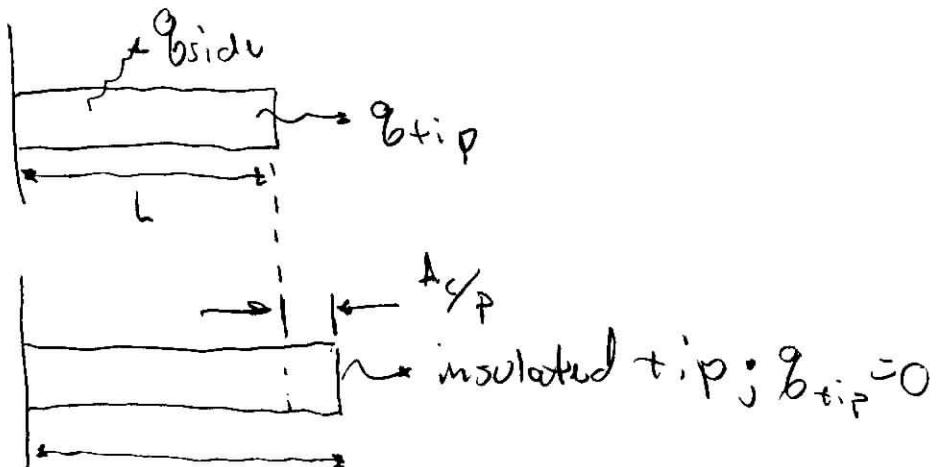
$$\boxed{L_{corr} = L + \frac{A_s}{P}} \quad \begin{matrix} \text{with} \\ \text{insulated tip} \end{matrix}$$
